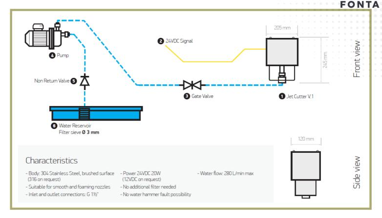
This superior cutting device stands out from all other interactive "water jet jumping" feature devices for its endurance and performance. Can cut so fast and so accurate - with the right nozzle, it can make small water balls to pop up!
